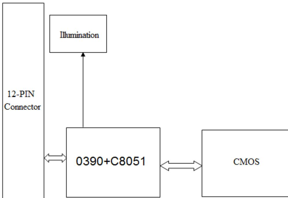
The engine connected with the host via the 12-pin FPC cable. For more details about the 12-pin FPC cable, please see **12-pin FPC** in Chapter 4.
